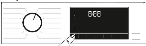
Whenever a new programme is selected, the recommended temperature for the programme appears on the temperature indicator. It is possible that the recommended temperature value is not the maximum temperature that can be selected for the current programme.
