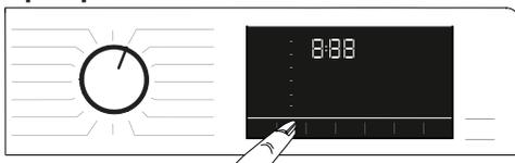
Whenever a new programme is selected, the recommended spin speed of the selected programme is displayed on the **Spin Speed** indicator.
