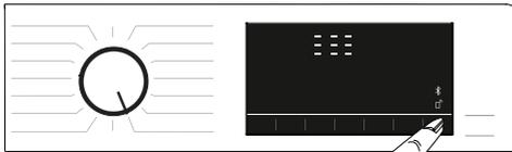
When the Remote Control is on, you can only manage, turn-off and status follow-up operations through your washing machine. And all functions except child lock can be managed through the application. You can follow whether the Remote Control function is On or Off through the function indicator on the button. If the Remote Control function is Off, all the operations are handled on the washing machine and only status follow-up is allowed on the application.
