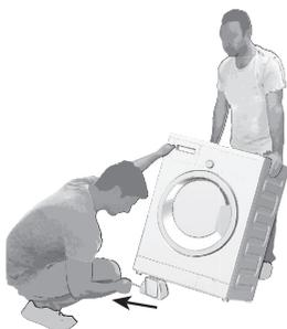
Tilt the machine backwards to remove the packaging reinforcement. Remove the packaging reinforcement that is attached to the ribbon. Do not attempt this operation alone, get help.
