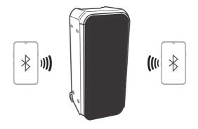
4 When two smartphones and the product are connected, the BT LED turns on.
