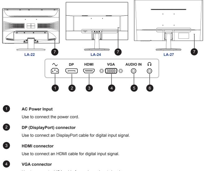
Use to connect a VGA cable for analogue input signal.
