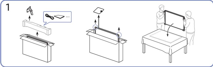
As shown in the figure, remove the product and foam cushion, and then place the product on the table with its front side facing the floor.
