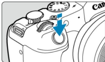
This activates autofocus and the automatic exposure system that sets the shutter speed and aperture value.
