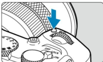
By pressing the <M-Fn> button once (or repeatedly) and then turning the <☀> or <☀> dial, you can set the white balance (☑), drive mode (☑), flash exposure compensation (☑), Picture Style (☑), metering mode (☑), AF operation (☑), ISO speed (☑), and AF area (☑).
