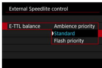
You can set your preferred appearance (balance) for flash shots. This setting enables you to adjust the ratio of ambient light to Speedlite light output.
