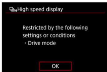
You can see the overriding function by selecting the dimmed menu item and pressing the  $\langle \text{Q} \rangle$  button.
