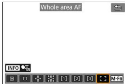
Uses auto selection AF in a whole-area AF frame to cover a larger area than Flexible Zone AF, which makes focusing easier than with 1-point AF/Expand AF area/Flexible Zone AF and effective for moving subjects.
