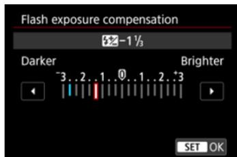
Just as exposure compensation is adjustable, you can also adjust flash output.
