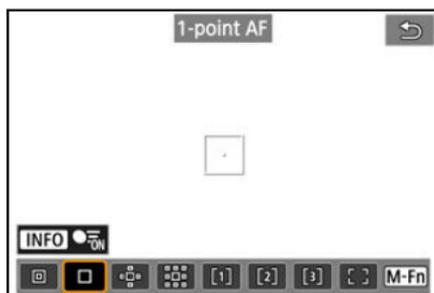
The camera focuses using a single AF point
