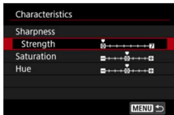
Adjust as needed. Select an option ([**Sharpness: Strength**], [**Saturation**], or [**Hue**]), adjust the effect level, then press the < (MENU) > button.
