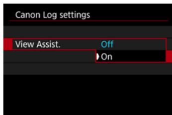
When played on the camera, these movies may look darker and have lower contrast than movies recorded with a Picture Style applied, due to Canon Log image characteristics, which are intended to ensure a wide dynamic range. For clearer display that makes it easier to check details, set **[View Assist.]** to **[On]**.
