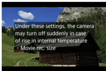
The guidance warns that the camera may become hot internally if movies are recorded under the current settings, and that if you continue recording, the camera may turn off automatically.
