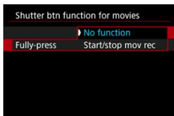
With **[Fully-press]** set to **[Start/stop mov rec]**, you can start/stop movie recording not only with the movie shooting button but also by pressing the shutter button completely, or by using Remote Switch RS-60E3 (sold separately).
