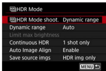
Suitable for landscape and still-life shots. For each shot, three images of different exposures (standard exposure, underexposure, and overexposure) are captured and automatically merged.
