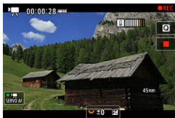
[REC] flashes in red if you continue recording after the indicator reaches level 9, marked in orange. A flashing icon indicates that the camera will soon turn off automatically.
