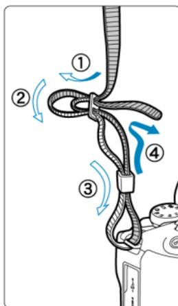
Pass the end of the strap through the strap mount from the bottom, then pass it through the strap buckle as shown. Pull the strap to take up any slack and make sure the strap will not loosen from the buckle.
