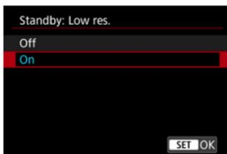
Set to **[On]** to conserve battery power and control the rise of camera temperature during standby.
