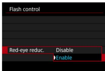
Set to **[Enable]** to reduce red-eye by firing the red-eye reduction lamp before firing the flash.
