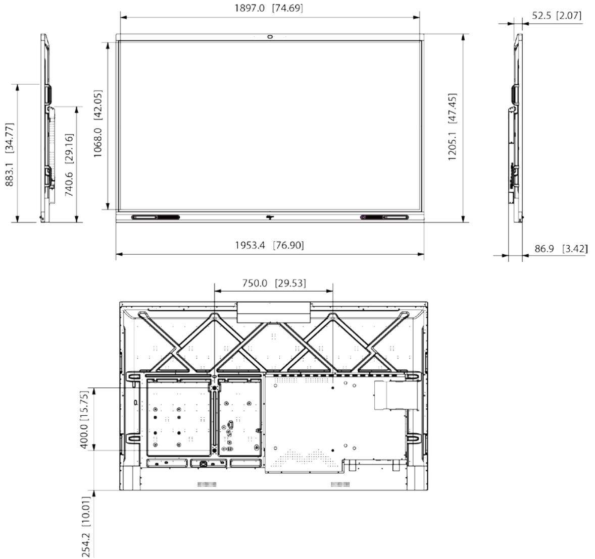
Figure 1-12 Dimensions (without camera: mm [inch])
