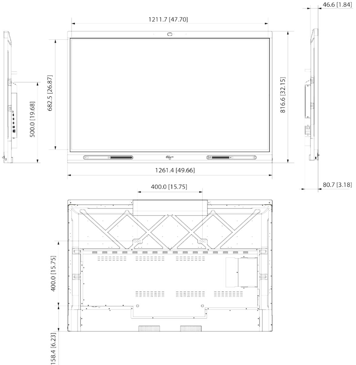
Figure 1-6 Dimensions (without camera: mm [inch])
