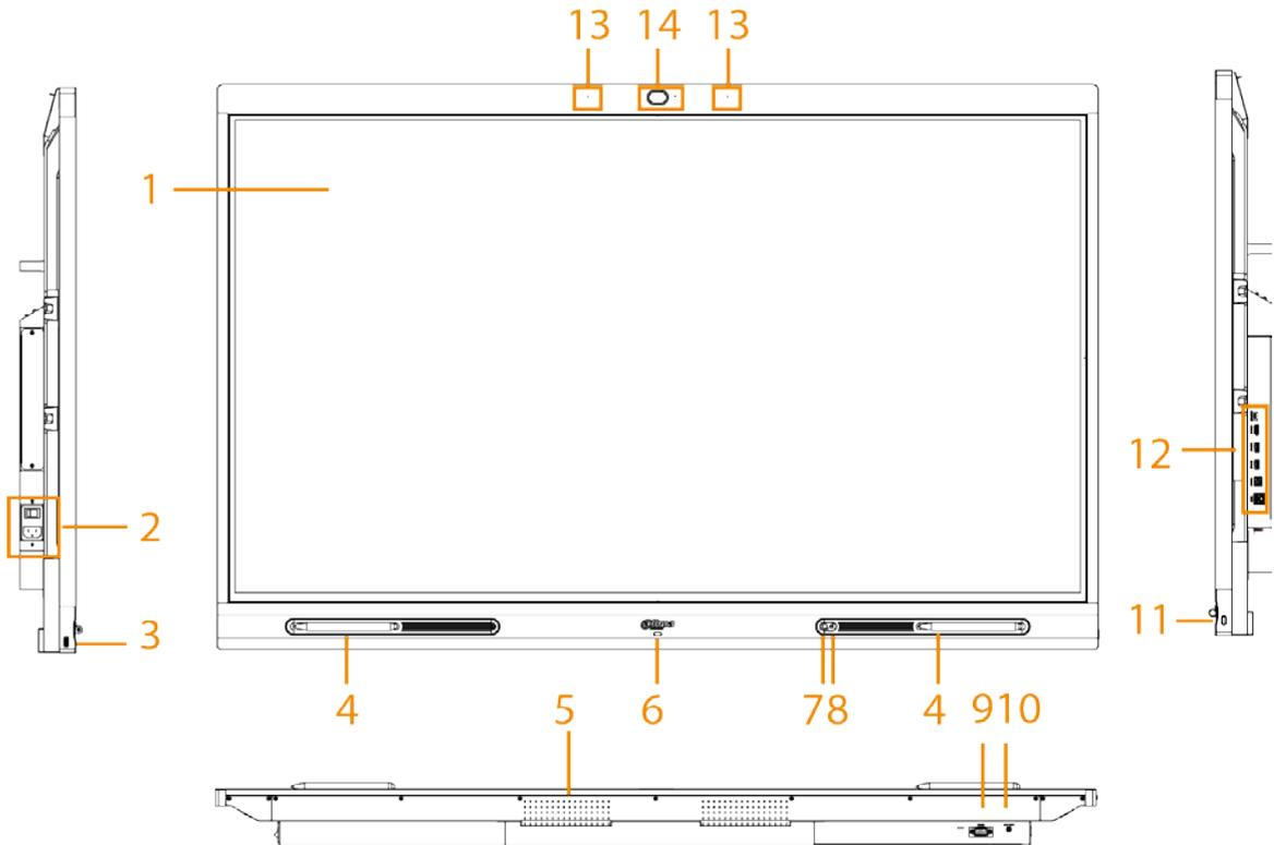
Figure 1-2 Appearance (55-inch series without camera)
