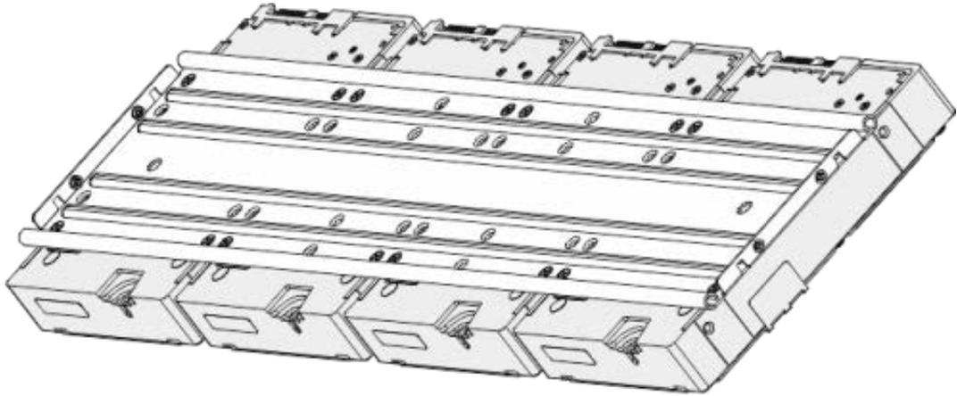
**Step 6** Lock the two HDD brackets.
