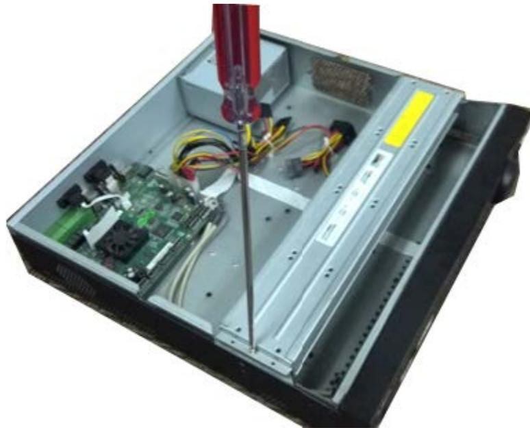
Step 2 Take off the bottom of the HDD bracket and CD-ROM bracket.
