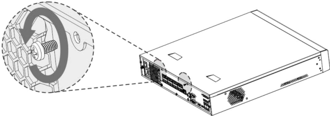
**Step 2** Remove the case cover along the direction shown in the following arrow.
