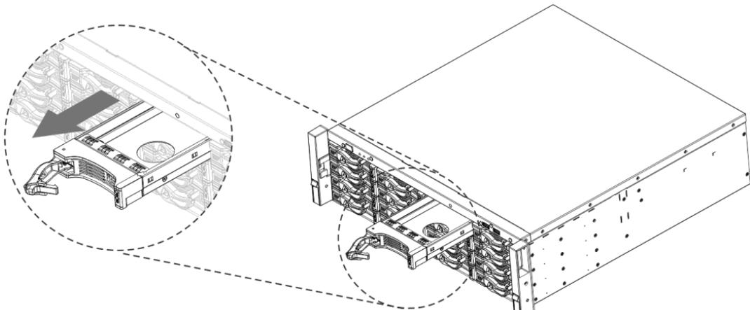
**Step 2** Put the HDD into the HDD box along the direction shown in the following arrow.
