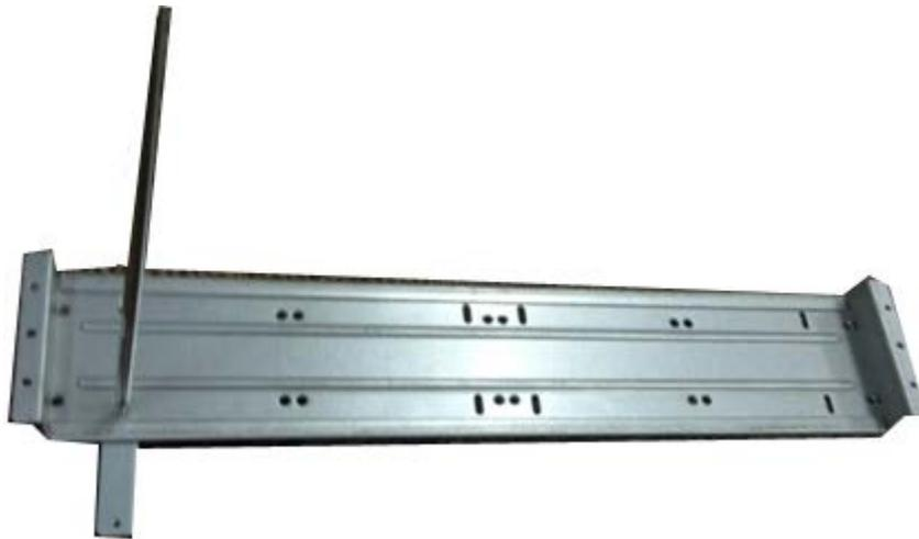
**Step 4** Install a pair of the CD-ROM bracket. Please make sure that the reverse side is secure too.
