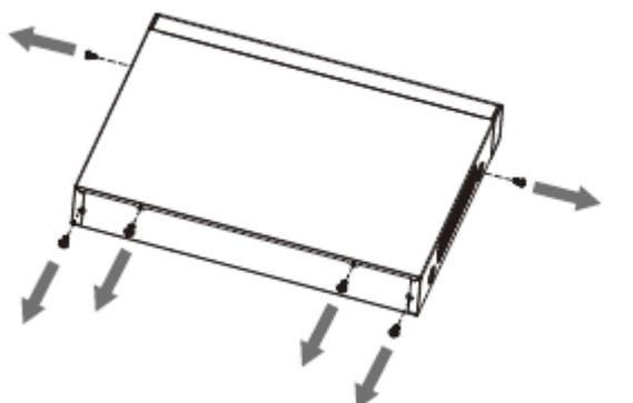
Step 2 Remove the cover in the direction of the arrow as shown in the figure below.
