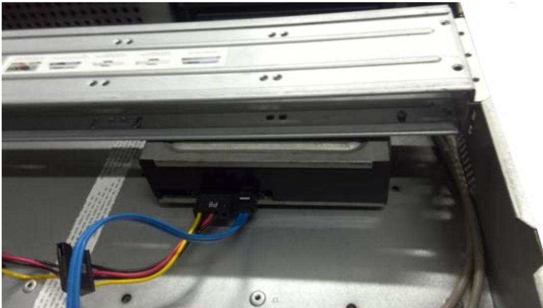
Step 9 Secure the HDD bracket and put the top cover back.
