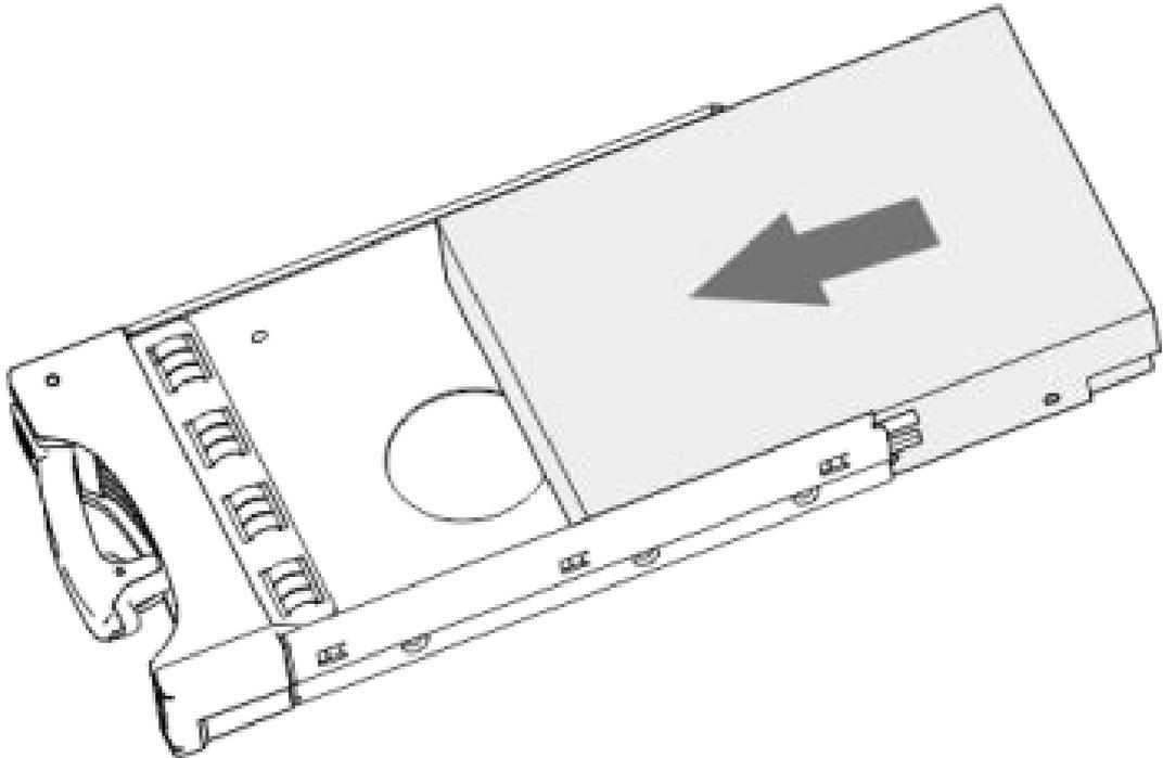
**Step 3** Fasten the screws on the sides of the HDD box.
