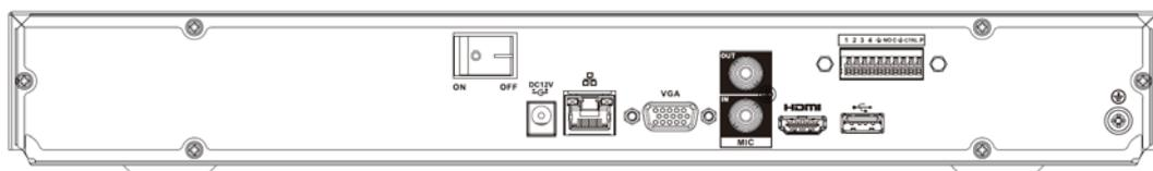
The NVR42-P-4KS2/NVR42-P-4KS2/L series rear panel is shown as below.
