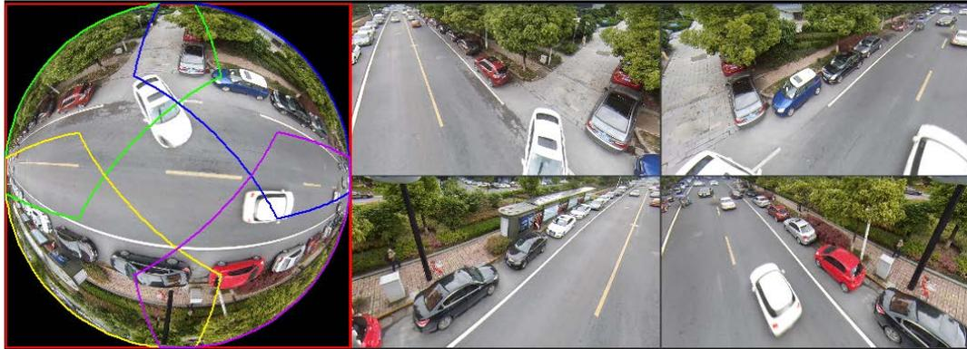
You can adjust the color pane on the left pane or use your mouse to change the position of the small images on the right pane to realize fish eye de-warp.
