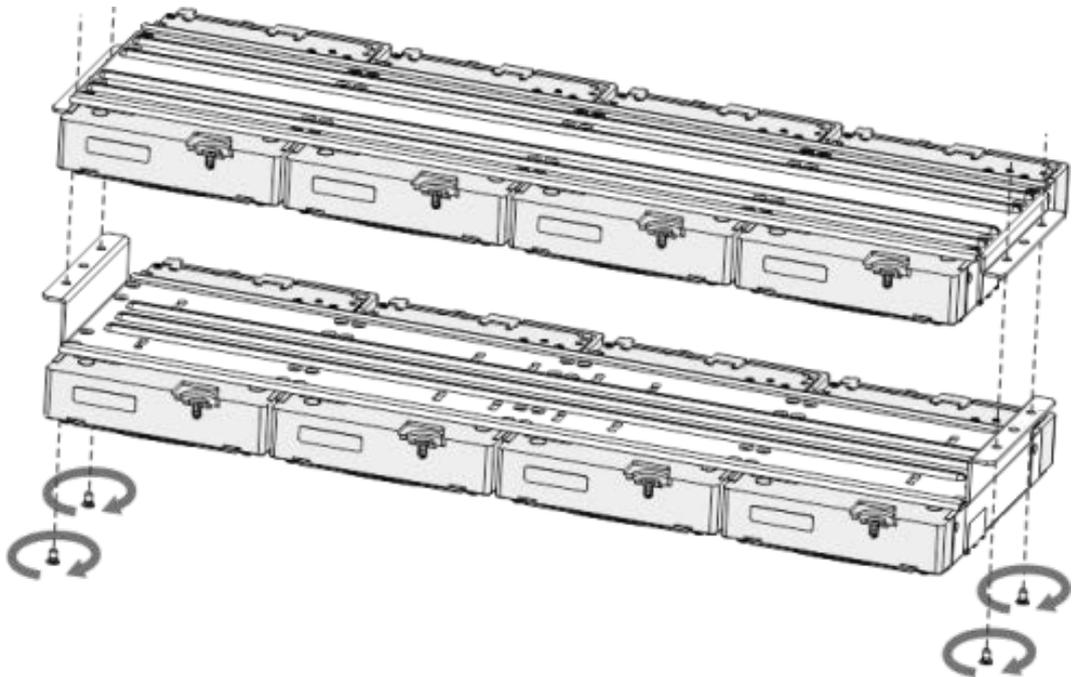
**Step 7** Place the bracket to the device and then fasten the screws on the sides of the bracket.
