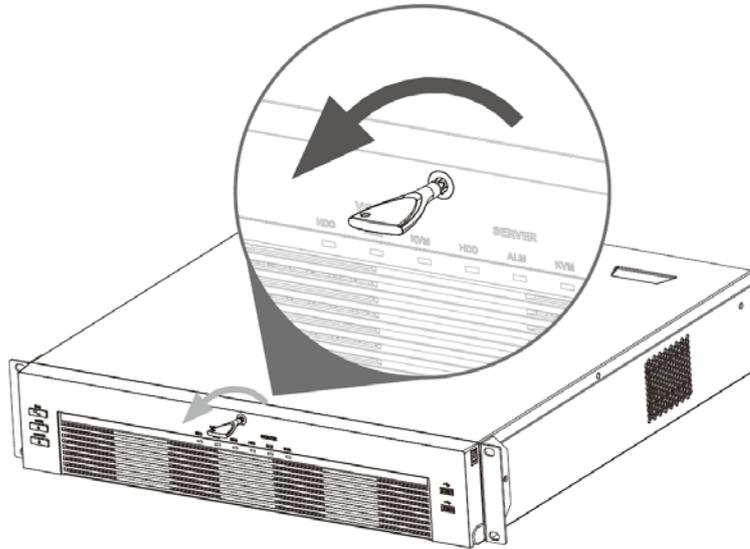
**Step 2** Press the button on the 2 sides to open the front panel.
