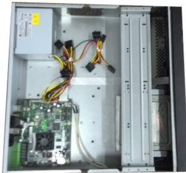
Step 8 Connect the SATA cable and power wire.
