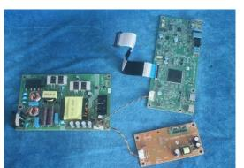
Remove the Mylar. Use a Philips-head screwdriver to remove 12 screws for unlocking the main board and the adapter board
