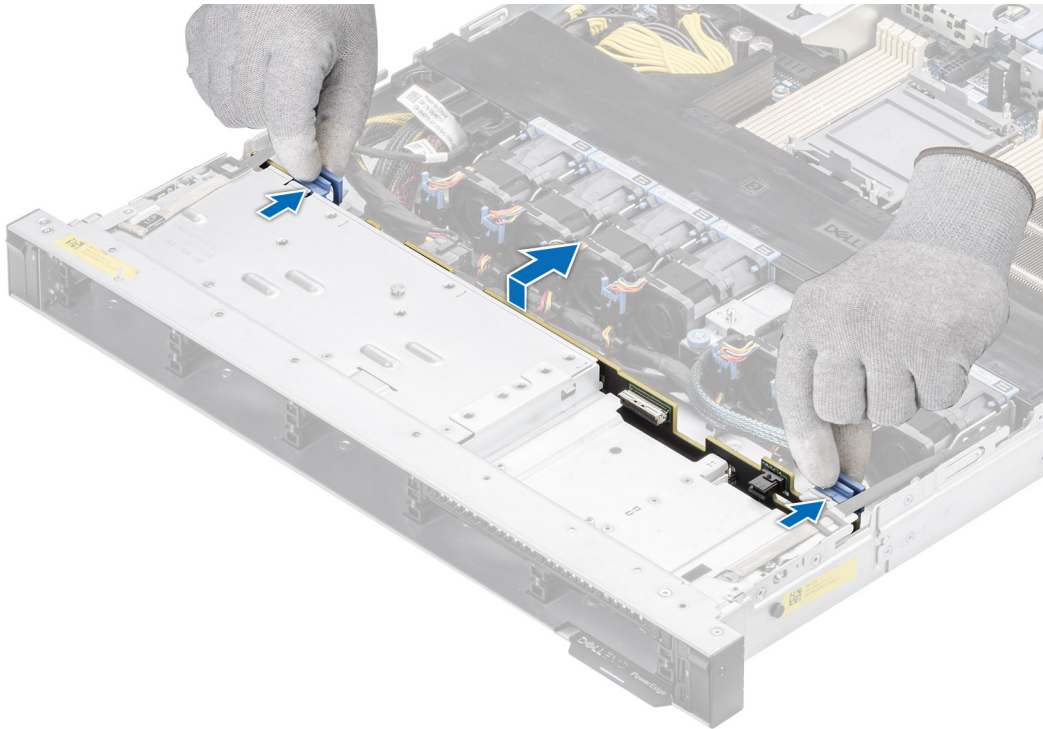
Figure 37. Removing the backplane
