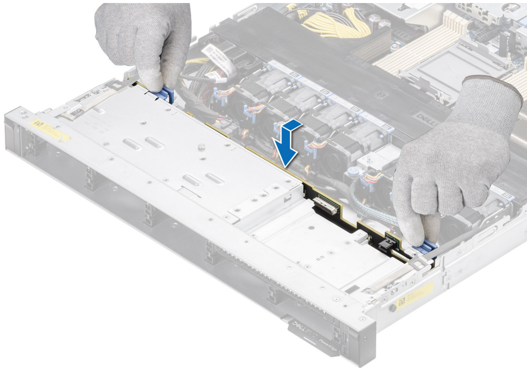
Figure 38. Installing the drive backplane
