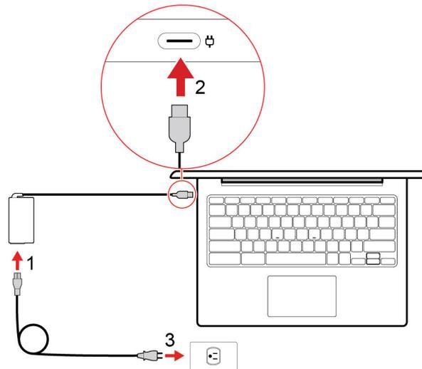
1. Connect the power cord to the ac power adapter.
