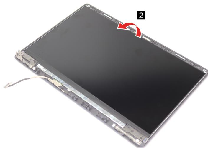
*Figure 18. Turn the LCD module*
