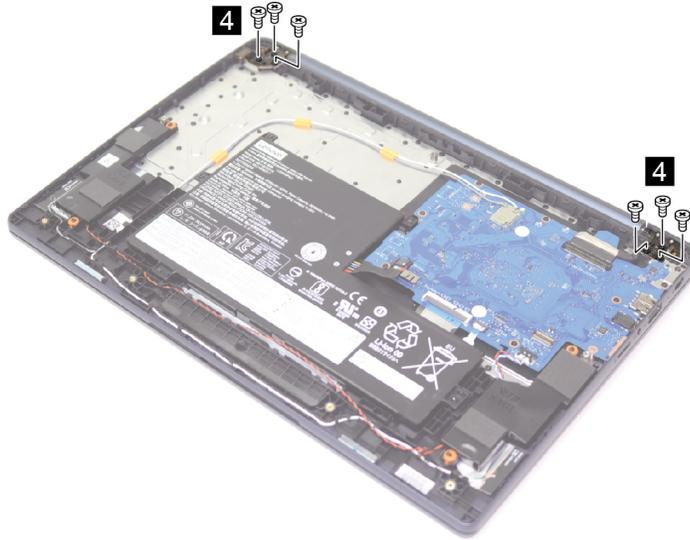
Figure 13. Remove six screws and open both hinges
