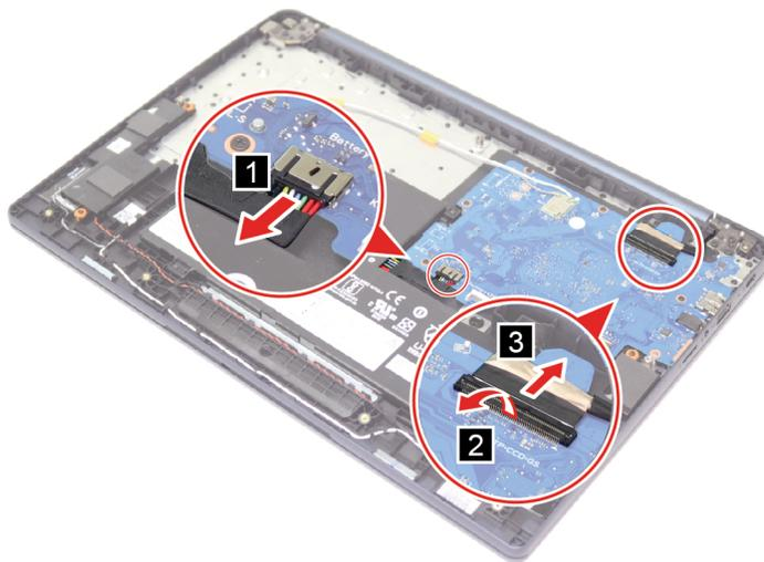
Figure 12. Disconnect the battery pack cable and EDP cable
