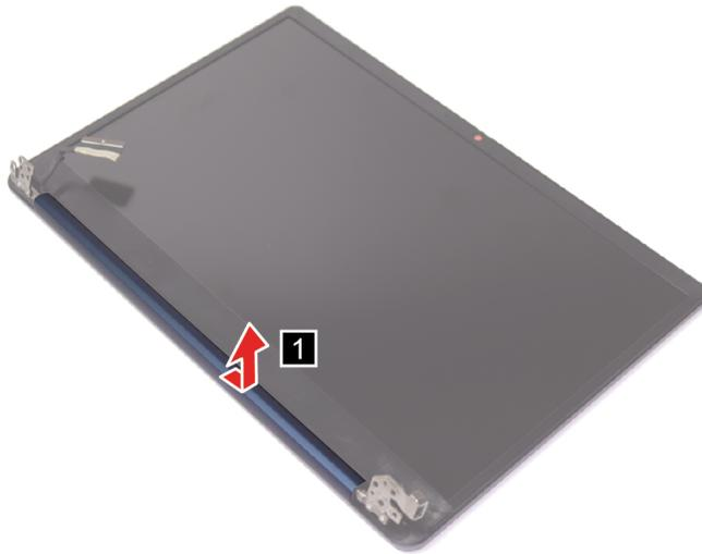
*Figure 15. Remove the hinge cover*
