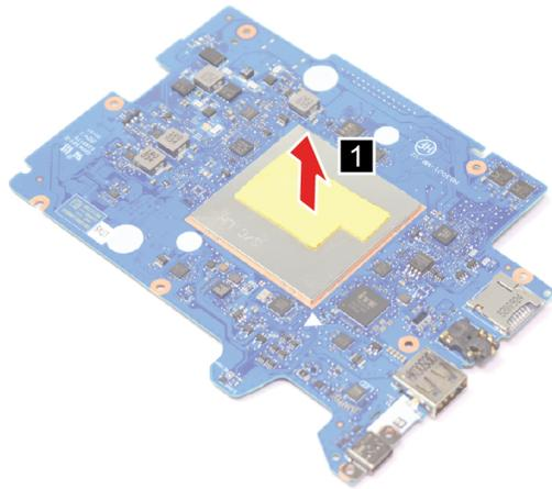
Figure 11. Remove the thermal pad
