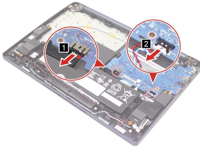
*Figure 4. Disconnect the battery pack cable and the speaker cable from the system board*
