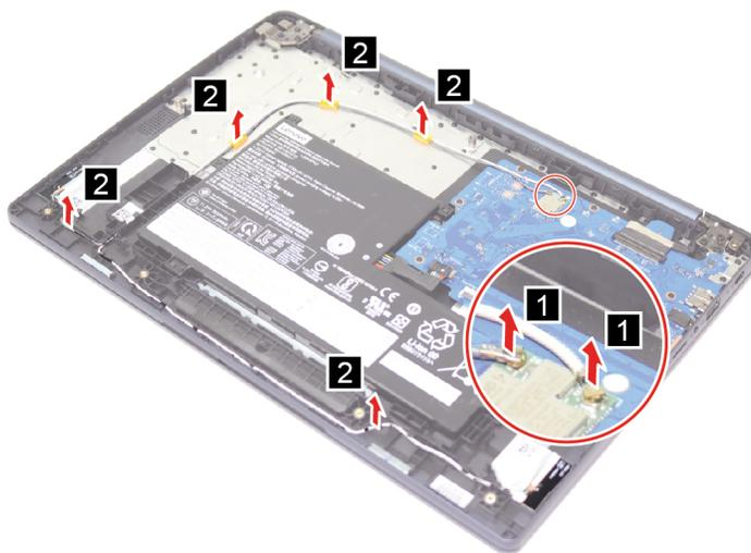
Figure 6. Remove the antenna
