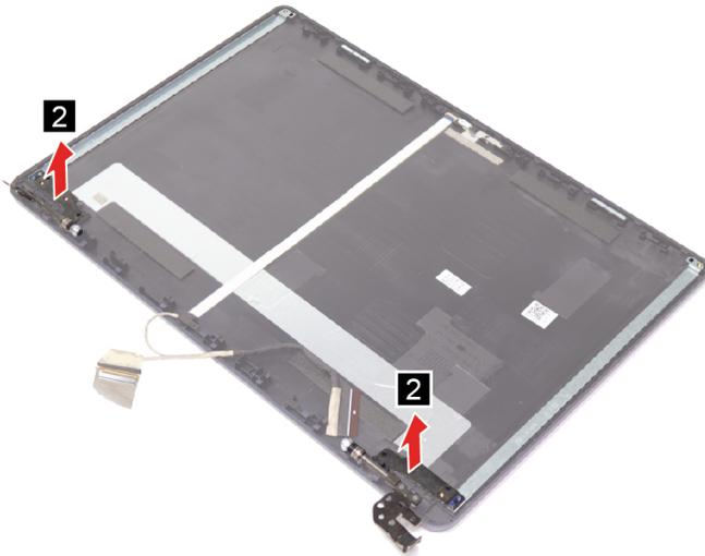
Figure 21. Remove the two hinges
