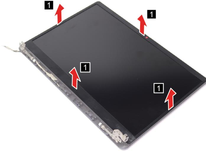
Figure 16. Remove the LCD bezel
