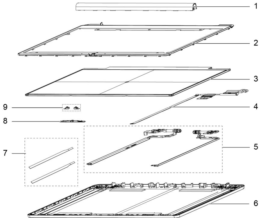
Figure 2. IdeaPad 3 Chrome 14M836 LCD exploded view
