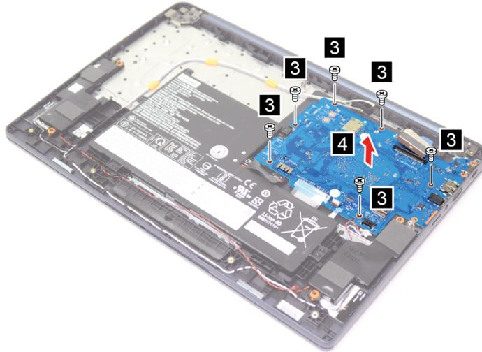
Figure 10. Remove six screws and remove the system board
