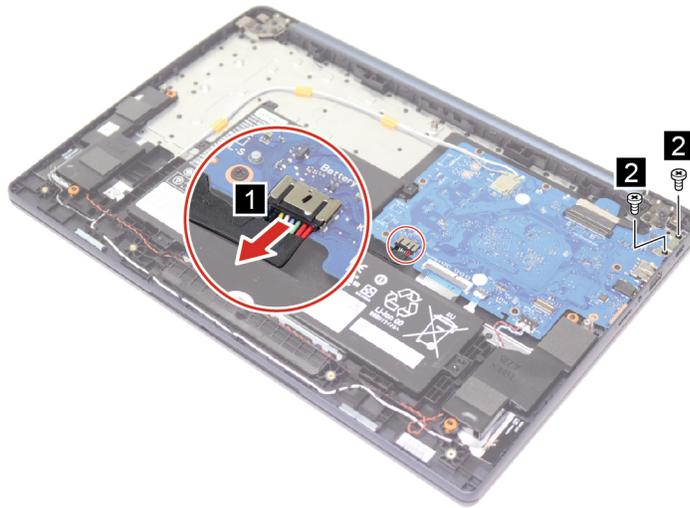
Figure 7. Remove the battery pack cable and then remove two screws
