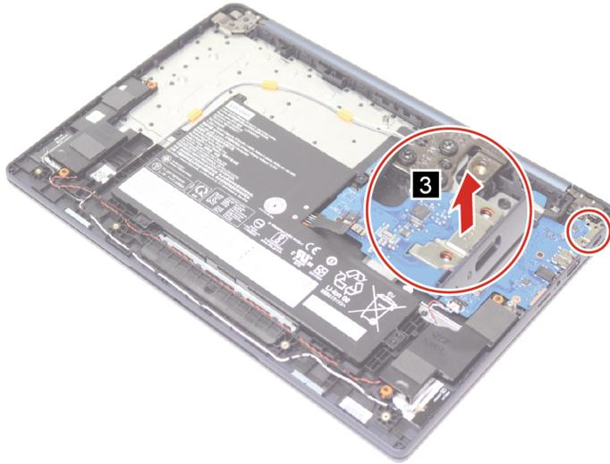
Figure 8. Remove the type-c bracket
