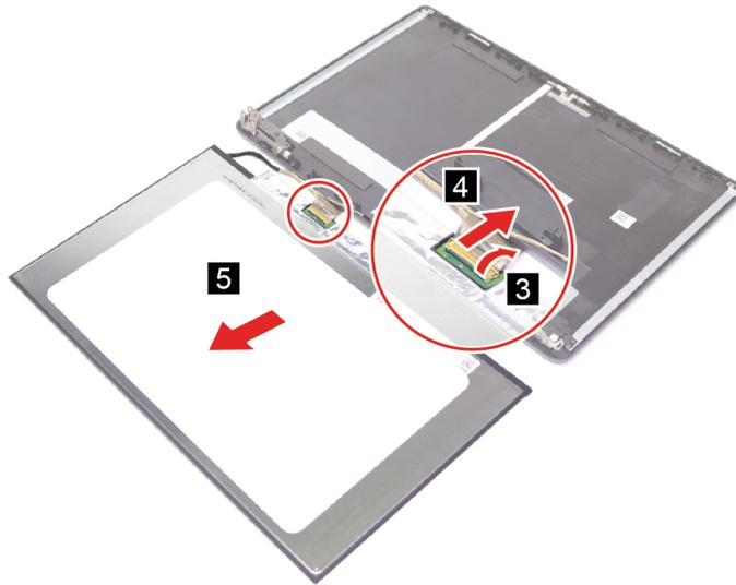
Figure 19. Disconnect the EDP cable and remove the LCD module.
