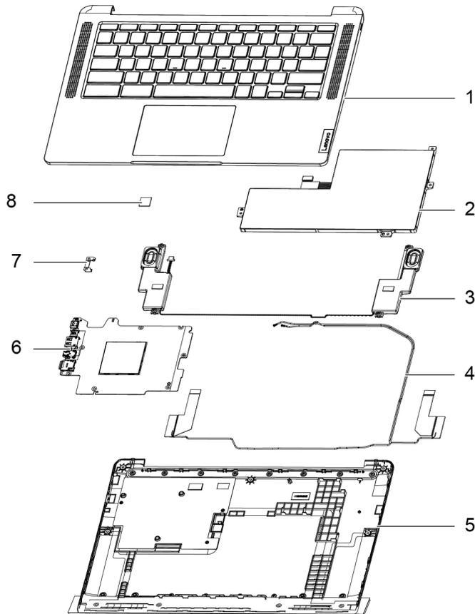
Figure 1. IdeaPad 3 Chrome 14M836 exploded view
