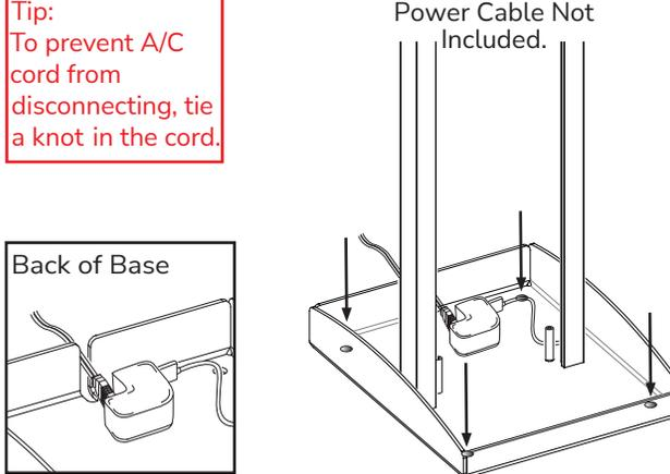
Route USB cable and plug into charging cube. Four 3/8" holes provided in the base for Floor Mounting
