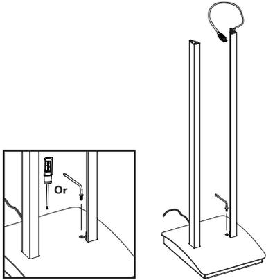
Secure Base Cover with M5 X 20mm Flat Head Torx Screw (H) using T-25 Torx Wrench(C).
