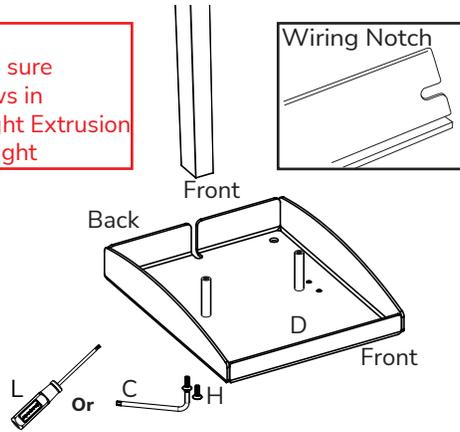
Locate the Upright Extrusions (D). Make sure extrusion has the flat edge facing forward. Install the M5 X20mm Flat Head Torx Screws (H) tighten using T-25 Torx Wrench (C).
