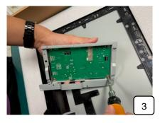
The frame deco can be removed by hand and screw driver.
