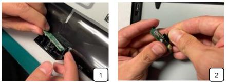
After removing tape and mylar, bracket can be easily removed. Then, the mainboard can be removed by screw driver.
