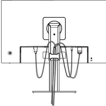
Rotate Set(Pivot) and put connectors. It is easy to put connectors and manage cables using cable holder.
