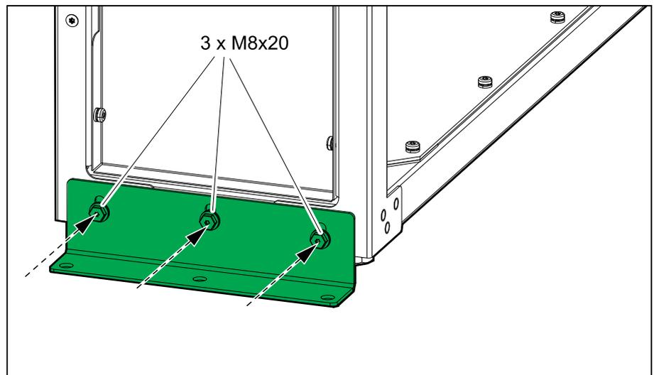
21. Mount the front and rear transportation brackets to the floor. Use appropriate hardware for the floor type - the hole diameter in the bracket is  $\varnothing 12$  mm. The requirement is M10 strength grade 8.8 hardware.
