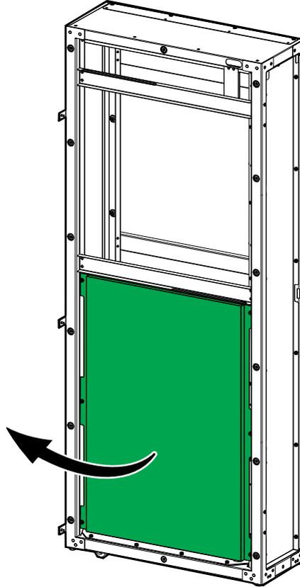
2. Install the lower side plate on the right side of the bottom entry cabinet.
