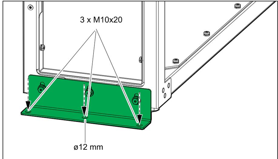
22. Reinstall the front plate on the bottom entry cabinet.
