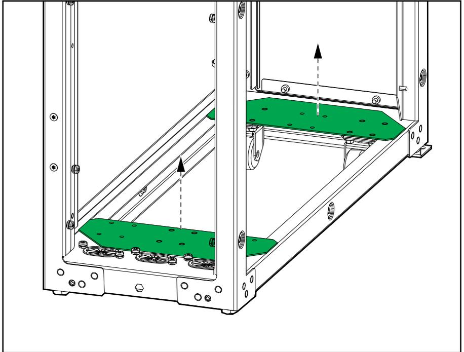
15. Drill/punch holes for cables or conduits/grommets in the gland plate. Install conduits/grommets (not provided), if applicable.
