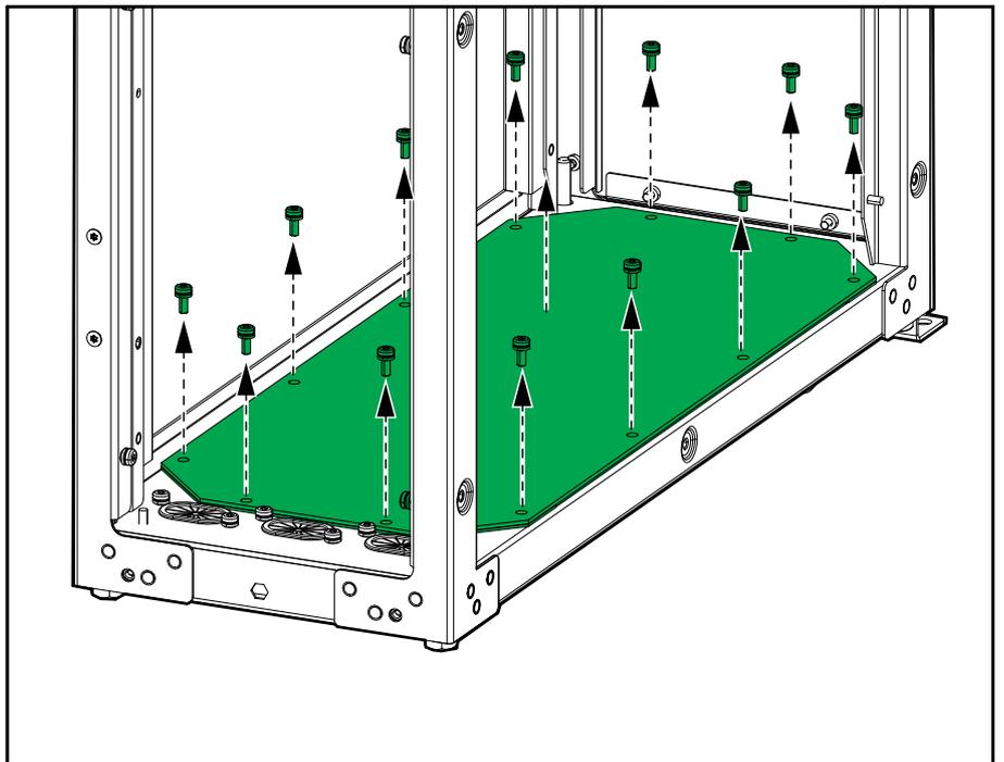
12. Remove the supporting plates with casters. Discard the supporting plates with casters.
