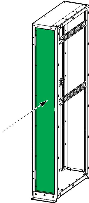
23. Install the left side panel on the bottom entry cabinet. The left side panel was removed from the UPS earlier.
