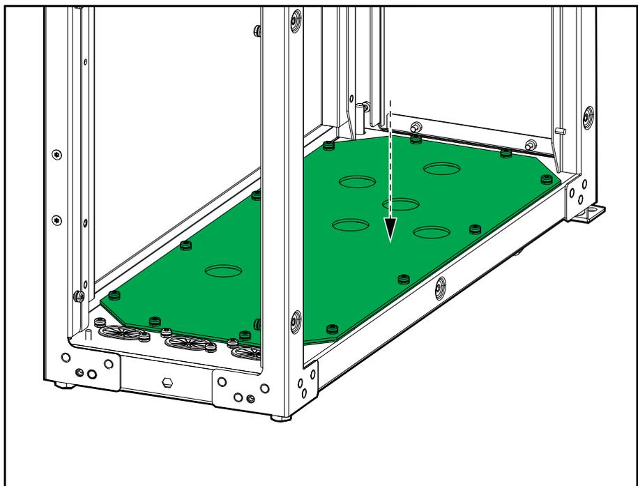
15. Remove the inner front plates and the rear panel from the UPS.
