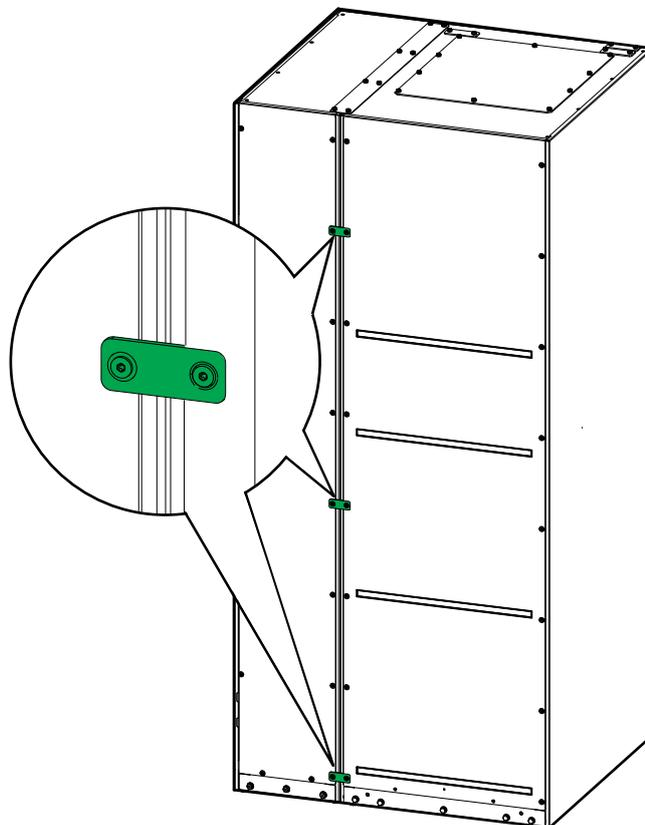
8. Remove the front plate from the bottom entry cabinet.
