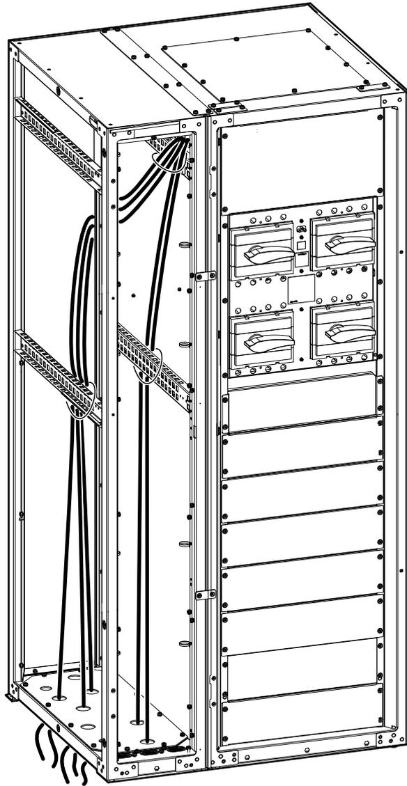
19. Route the signal cables up through the bottom entry cabinet and into the UPS. Route as shown to separate the Class 2/SELV cables from the non-Class 2/non-SELV cables.
