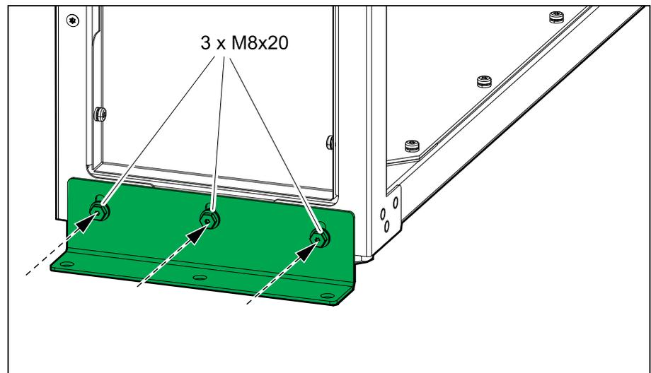
19. Mount the front and rear transportation brackets to the floor. Use appropriate hardware for the floor type - the hole diameter in the bracket is  $\varnothing 12$  mm. The requirement is M10 strength grade 8.8 hardware.
