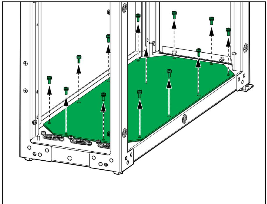
14. Remove the supporting plates with casters. Discard the supporting plates with casters.
