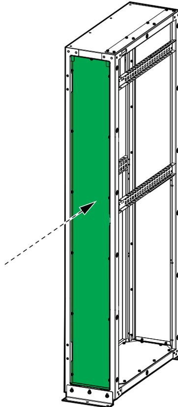
21. Install the right side panel on the bottom entry cabinet. The right side panel was removed from the UPS earlier.
