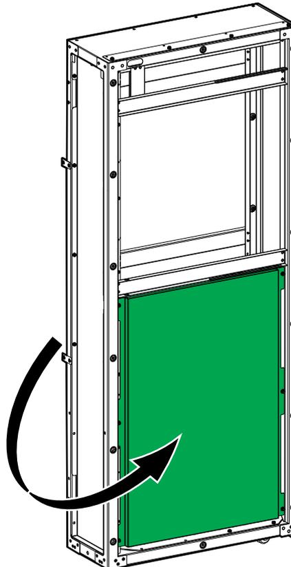
3. Remove the left side panel from the UPS. Save for installation on the bottom entry cabinet.
