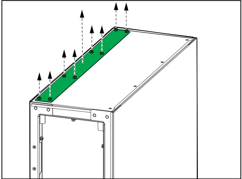
5. Install the top interconnection bracket between the UPS and the bottom entry cabinet.
