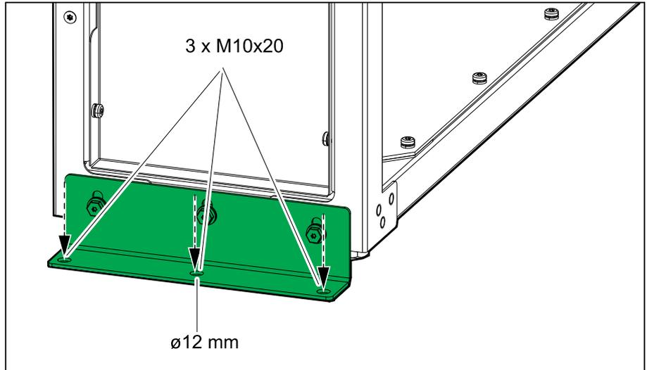
20. Reinstall the front plate on the bottom entry cabinet.
