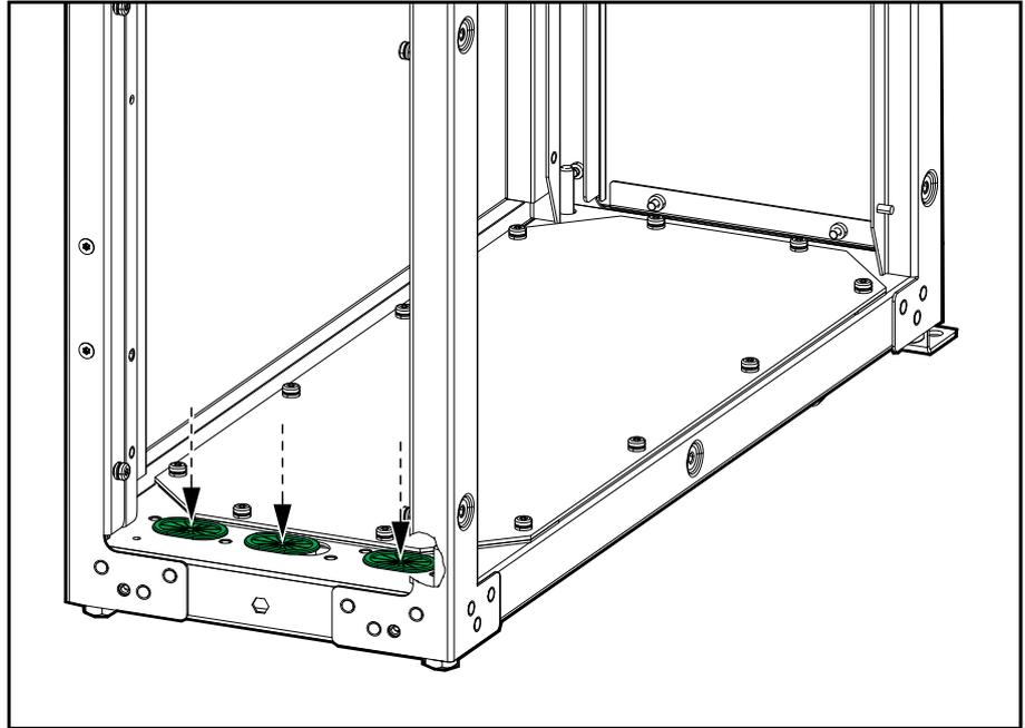
13. Remove the bottom gland plate and the supporting plates.
