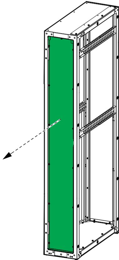
11. Remove the plates for the signal cables.
