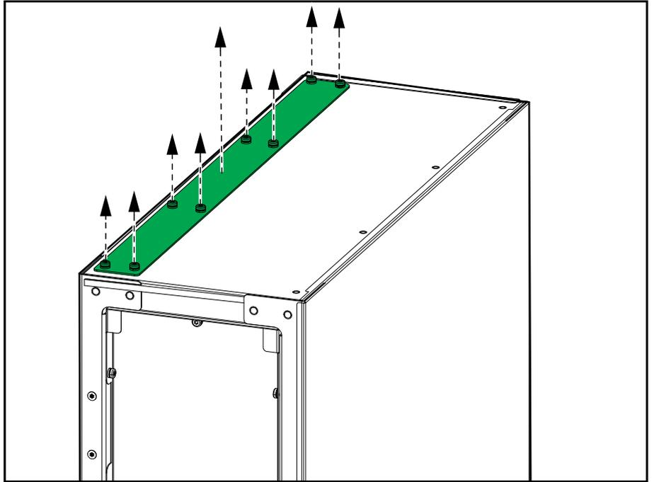
7. Install the top interconnection bracket between the UPS and the bottom entry cabinet.
