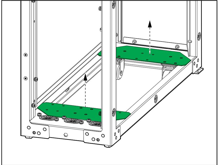
13. Drill/punch holes for cables or conduits/grommets in the gland plate. Install conduits/grommets (not provided), if applicable.
