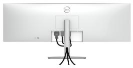
After attaching all necessary cables to your monitor and computer, (See Connecting your monitor for cable attachment) organize all cables as shown above.
