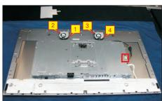
Tear off three pieces of VBH tape on the specific position as the picture below shown. Disconnect the function key cable from the connector of the interface board. Use a Philips-head screwdriver to remove eight screws for unlocking the middle iron bezel with the panel module. Remove the middle iron bezel.
