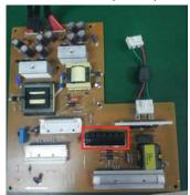
S1 -1 Cut the glue between bulk cap. and PCB with a knife
