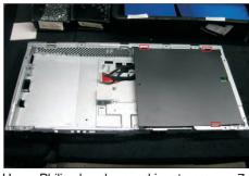
Use a Philips-head screwdriver to remove 7 screws for unlocking the power board and AC board, then remove the two boards from the hooks of the bracket chassis. Disconnect all of the cables.
