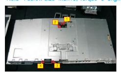
Turn over the bracket chassis. Use a Philips-head screwdriver to remove 4 screws for unlocking the interface board and LED driver board. Disconnect the cables of the interface board and LED driver board away from the power board, then remove the two board from the hooks of the bracket.
