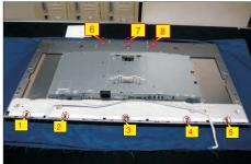
Use a Philips-head screwdriver to remove four screws for unlocking the bracket with the panel module. Use a Jip to lift up the bracket, then tear off the black mylar tape for releasing the LVDS connectors. Disconnect the LVDS cables from the connectors of the panel module.
