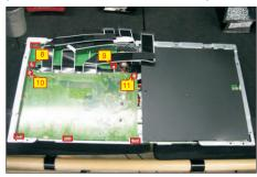
S15 Remove the Mylar from the hooks of the bracket chassis module.
