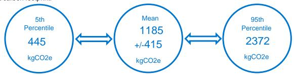
Carbon footprint calculations have a wide range based on a variety of factors including how the device is configured, where it was manufactured and more. Dell Technologies reports the 5th and 95th percentile of the carbon footprint estimate to reflect that uncertainty. For this product, that estimate has a mean of 1185 kg of CO2e and standard deviation of 415 kg of CO2e.
