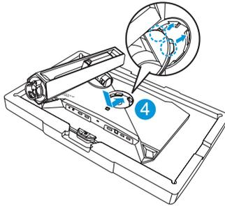
5. Align and install the base to the stand.
