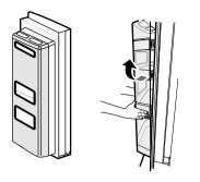
**2** Lift up and remove the baskets from the door in door casing.
