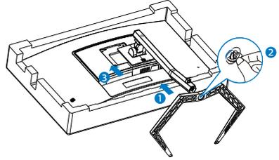
3. After attaching the base, erect the monitor with both hands on holding the monitor together with styrofoam firmly. Now you can pull out the styrofoam. When you pull out the styrofoam, do not squeeze the panel to avoid broken panel.
