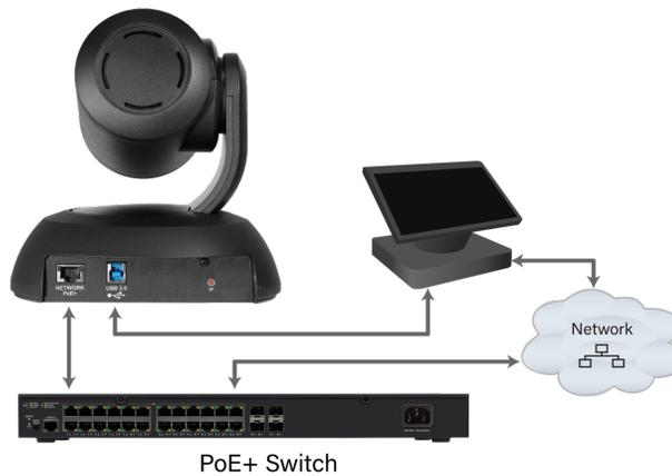
The PoE+ switch is not required. You can connect the camera to the network and to power using the mid-span power injector included with the camera.
