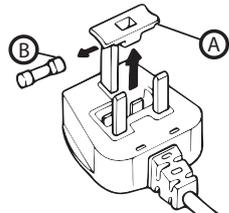
1. Remove the fuse cover (A) and fuse (B).
