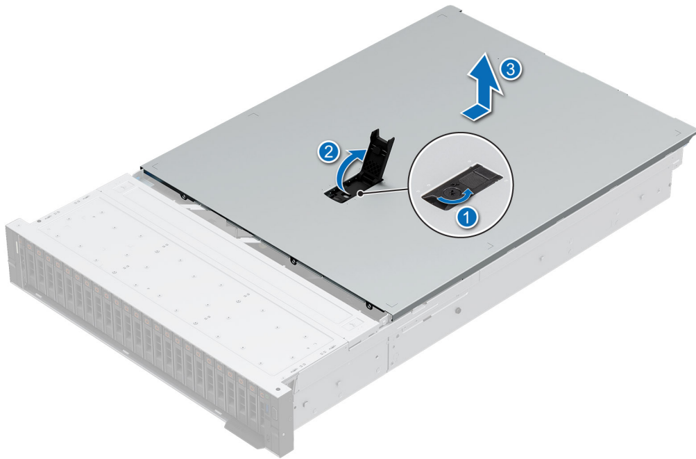
Figure 31. Removing the system cover
