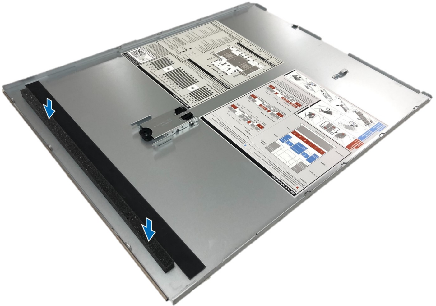
Figure 256. Installing Mylar foam on the system cover
