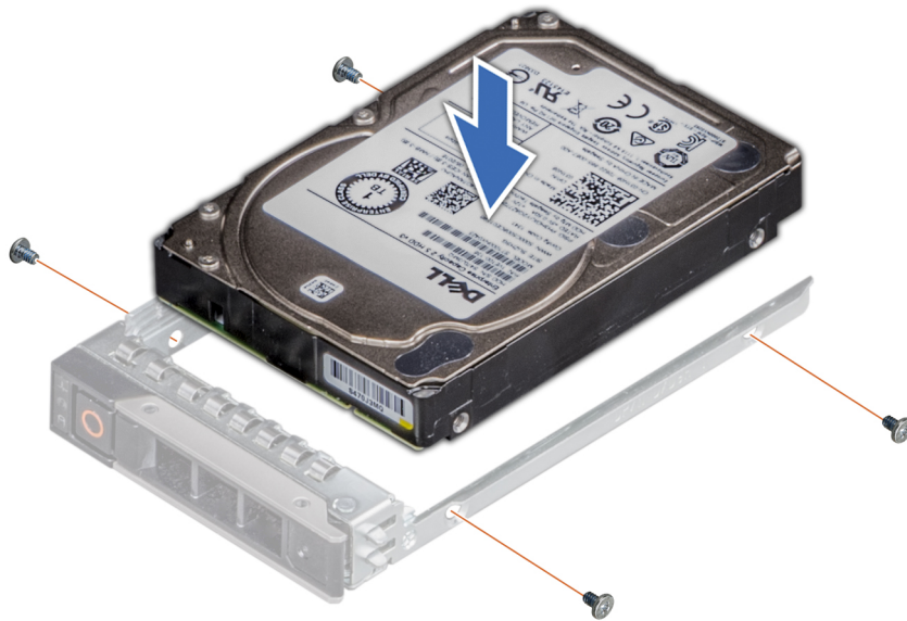
Figure 69. Installing a drive into the drive carrier
