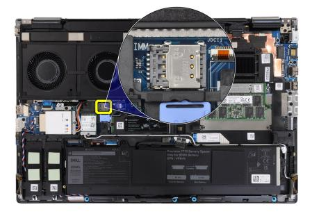
**CAUTION:** The SIM card cover is fragile and can be damaged if it is not properly unlocked before opening.
