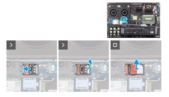
1. Gently slide the SIM card cover towards the left side of the SIM card slot to unlock the SIM card cover.
