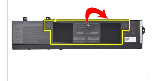
**3.** Flip the battery and peel the adhesive on the battery cable.
