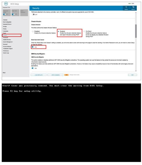
If Block Boot Until Cleared is set to OFF, select Continue to boot normally or BIOS-Setup to clear the alert.
