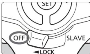
The wireless selector is for switching between normal flash shooting and wireless flash shooting. For normal flash shooting, be sure to set the wireless selector to <OFF>.
