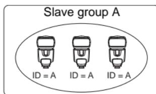
For example, if you have the slave ID set to <A> for three Speedlites, all three Speedlites will be controlled as if they were one Speedlite in slave group A.
