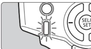
If the lens focal length blinks on the LCD panel, the periphery of the flash picture may turn out dark. Use the built-in wide panel (p.18).
