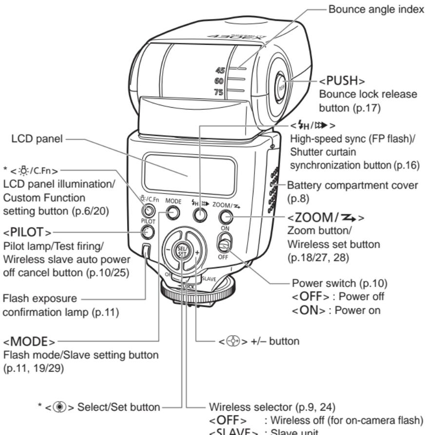
Asterisked buttons have a timer that keeps the button's function active for 8 sec. (8) after you let go of the button. The <LCD> illumination lasts for 12 sec.
