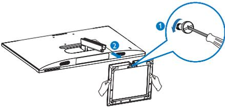
3. Remove the hinge cover from monitor body by using your fingers.
