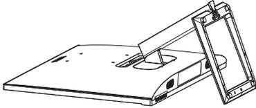
2. Use a screwdriver to loosen the screw located at the bottom of the base, and remove the base from the stand.
