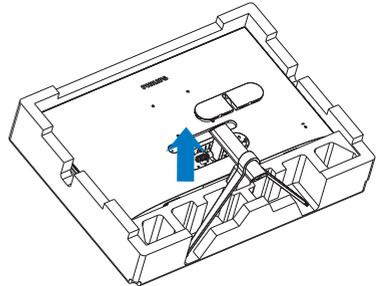
3. Use a screwdriver to remove the screws on the arm, and then detach the arm/stand from the monitor.
