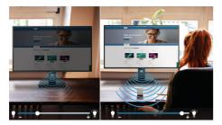
PowerSensor is a built-in 'people sensor' that transmits and receives harmless infrared signals to determine if user is present and automatically reduces monitor brightness when user steps away from the desk, cutting energy costs by up to 65 percent and prolonging monitor life
