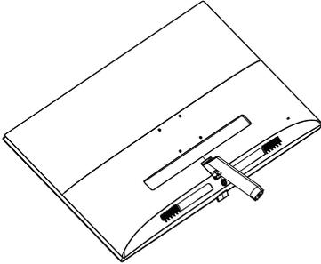
2. Hold the base stand with both hands and firmly insert the base stand into the base column.
