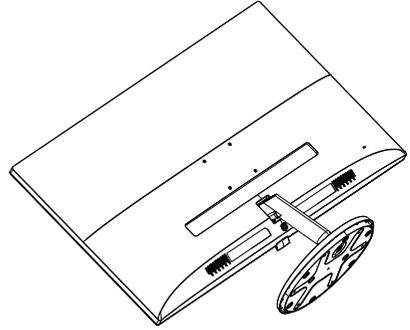
2. (1) Use screwdriver to loosen the screw located at the bottom of the base.
