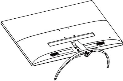
2. (1) Use screwdriver to loosen the screw located at the bottom of the base.
