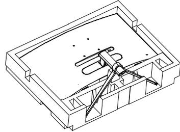
2. Remove the hinge cover from monitor body by using your fingers.
