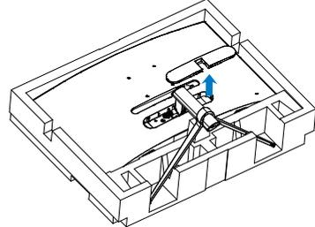
3. Use a screwdriver to remove the screws on the arm, and then detach the arm/stand from the monitor.
