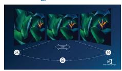
IPS displays use an advanced technology which gives you extra wide viewing angles of 178/178 degree, making it possible to view the display from almost any angle - even in 90 degree Pivot mode! Unlike standard TN panels, IPS displays gives you remarkably crisp images with vivid
