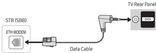
Connect the **DATA** port of the TV to the **ETH MODEM** port of the STB (SBB) with the Data cable.
