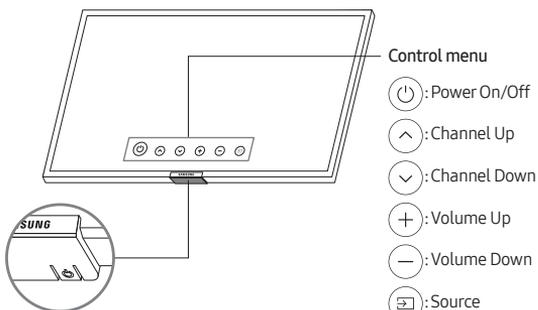
TV Controller button / Remote control sensor
