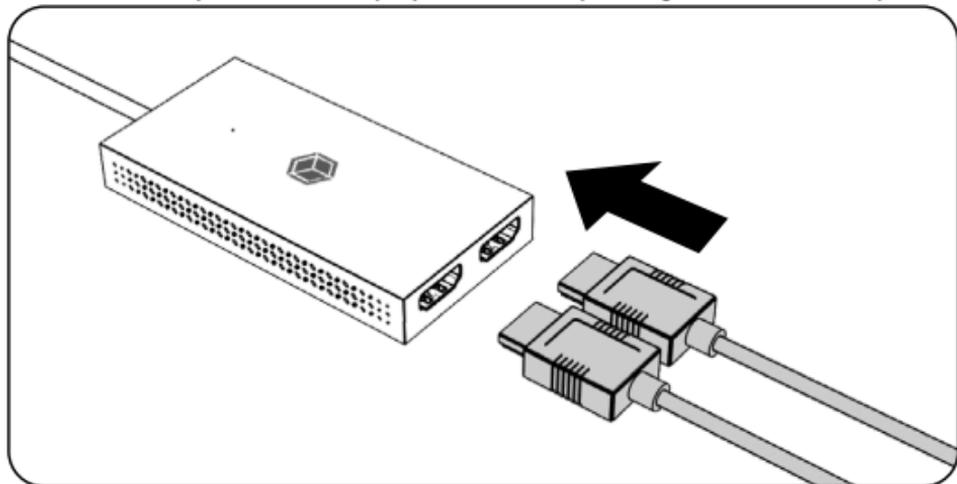
To use this splitter to its full potential, ensure that the host USB port of your computer supports **USB 3.2 Gen 1**.
