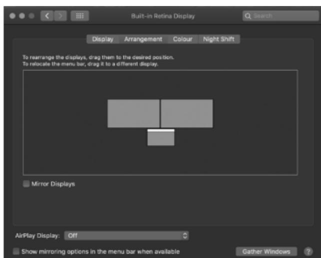
To set up scaled resolutions of the monitor displays, click the **Display** tab. In the window that now opens for the respective display, you can set your desired resolutions separately. Select the option **Scaled** and then select the appropriate size in the field below.
