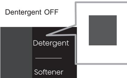
The detergent is turned off and will not be dosed at the end of the program. This is visible on the display as in the picture below. No LED indications.
