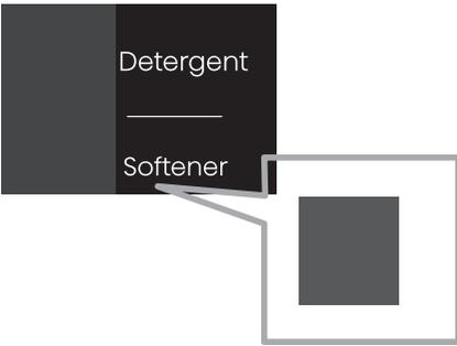
The softener is turned off and will not be dosed at the end of the program. This is visible on the display as in the picture below. No LED indications:
