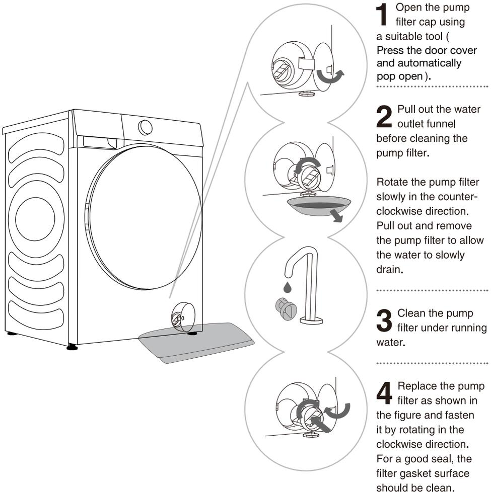
☼ The pump filter must be timely cleaned, especially after washing very fleecy, woolly, or very old laundry.
