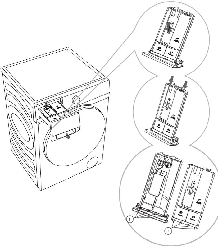
1. Open the detergent compartment, press the limit lever as shown in the figure, and pull out the detergent compartment;
