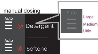
It is possible to manually select the desired amount of detergent dosage. We can set the desired dosage value of the detergent ourselves. There are three levels, little, medium and large. Manual dosing is selected when the Auto icon is not ON and lines can be selected (little, middle, large).
