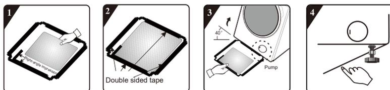
1. Before installing the noise reduction board, align and paste the acoustic absorption wool with and along the right-angle impression on bottom plate (this procedure is unnecessary for some of the models without acoustic absorption wool).
