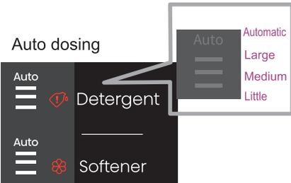
If the Auto icon is ON and all 3 lines are ON, it means that you have selected the automatic dosing function. The fabric detergent is dosed automatically, depending on how much laundry is in the drum.
