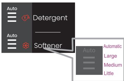
If the Auto icon is ON and all 3 lines are ON, it means that you have selected the automatic dosing function. The fabric softener is dosed automatically, depending on how much laundry is in the drum.
