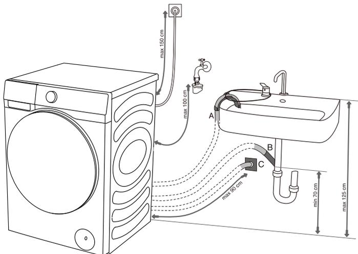
**C** Discharge hose can also be attached to a wall drain with a trap; such trap should be properly installed to allow cleaning.
