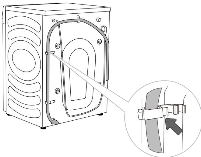
**D** The discharge hose has to be attached and affixed to the pin on the back of the washing machine, as shown in the figure. Max.
