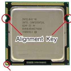
Yellow triangle is the Pin 1 indicator
