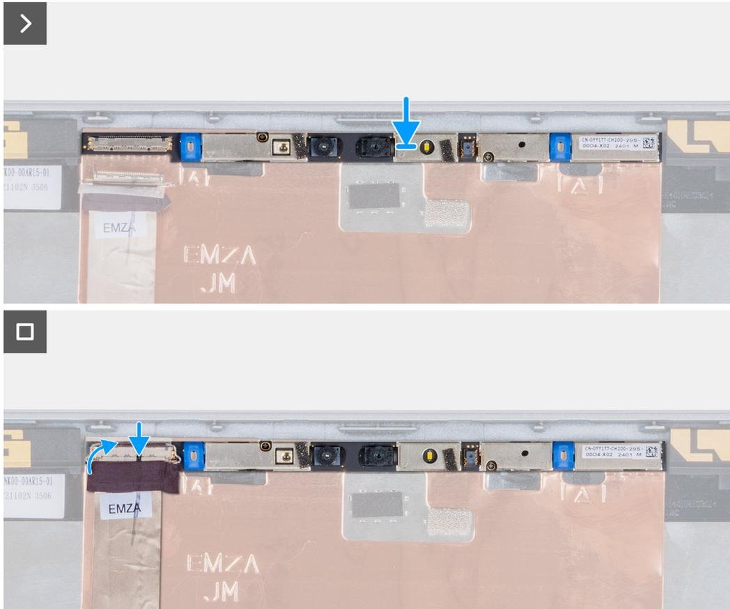
**Figure 3. Installing the camera module**
