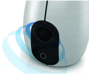
Bass-reflex acoustic load uses a bass pipe tuned to the acoustic volume of the speaker box, in order to reproduce deep bass from compact enclosures. The carefully designed profiled bass-pipe helps air flow and allows for deep and impactful bass, even at loud volumes while minimizing air turbulence that may cause distortion.
