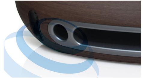
Bass-reflex acoustic load uses a bass pipe tuned to the acoustic volume of the speaker box, in order to reproduce deep bass from compact enclosures. The carefully designed profiled bass-pipe helps air flow and allows for deep and impactful bass, even at loud volumes while minimizing air turbulence that may cause distortion.
