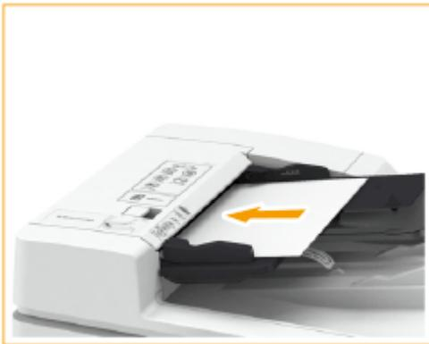
⇒ When insertion depth is sufficient, the Original Set Indicator lights up (imageRUNNER 2945i only).
