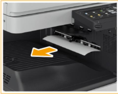
**3 Check whether paper is jammed in the output area or reversing unit.**
