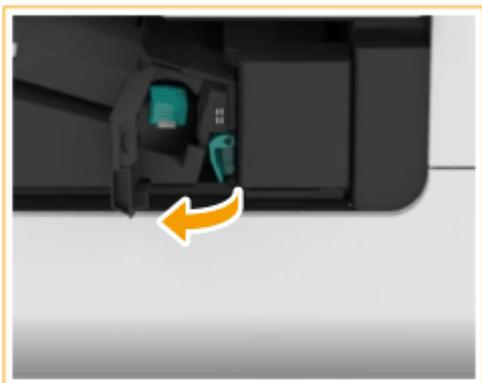
**4** Hold the lever ( **a** ), and slide the inner finisher to the left.
