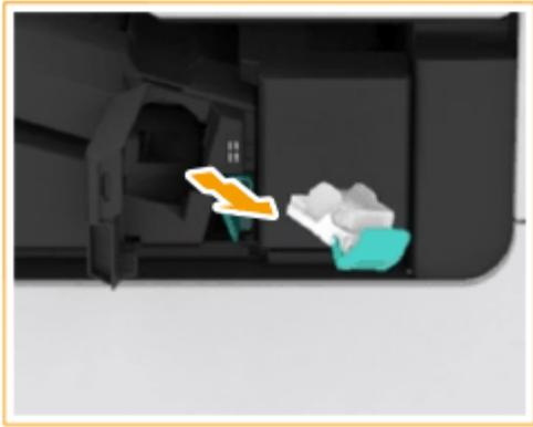
**4 Remove the jammed staple(s) from the staple cartridge.**
