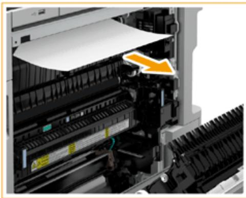
**4 Check whether paper is jammed in the fixing assembly.**
