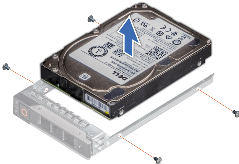
Figure 70. Removing the drive from the drive carrier
