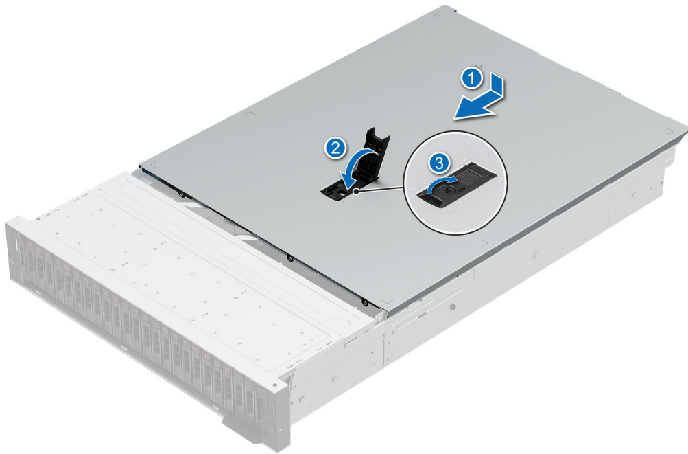
Figure 35. Installing the system cover
