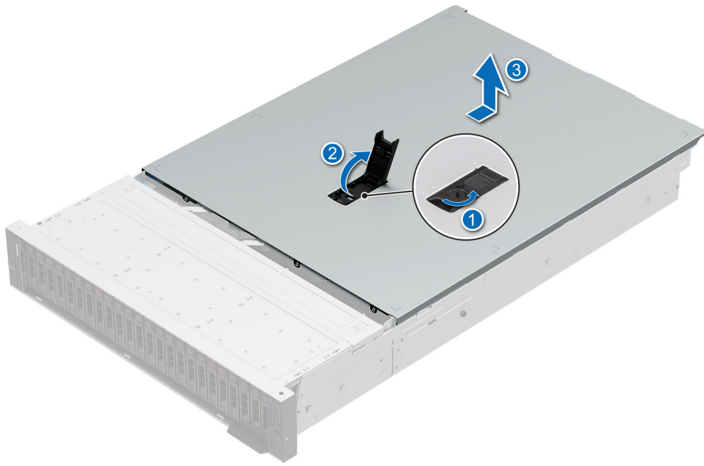
Figure 34. Removing the system cover
