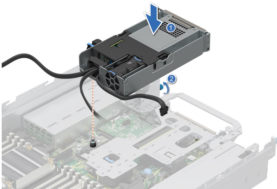
Figure 80. Installing the 4 x EDSFF E3.S rear drive module
