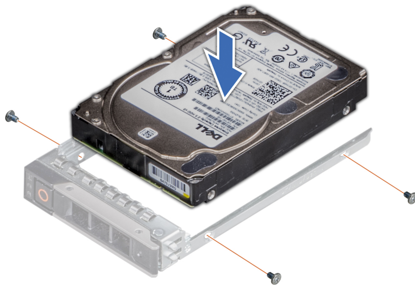
Figure 57. Installing a drive into the drive carrier
