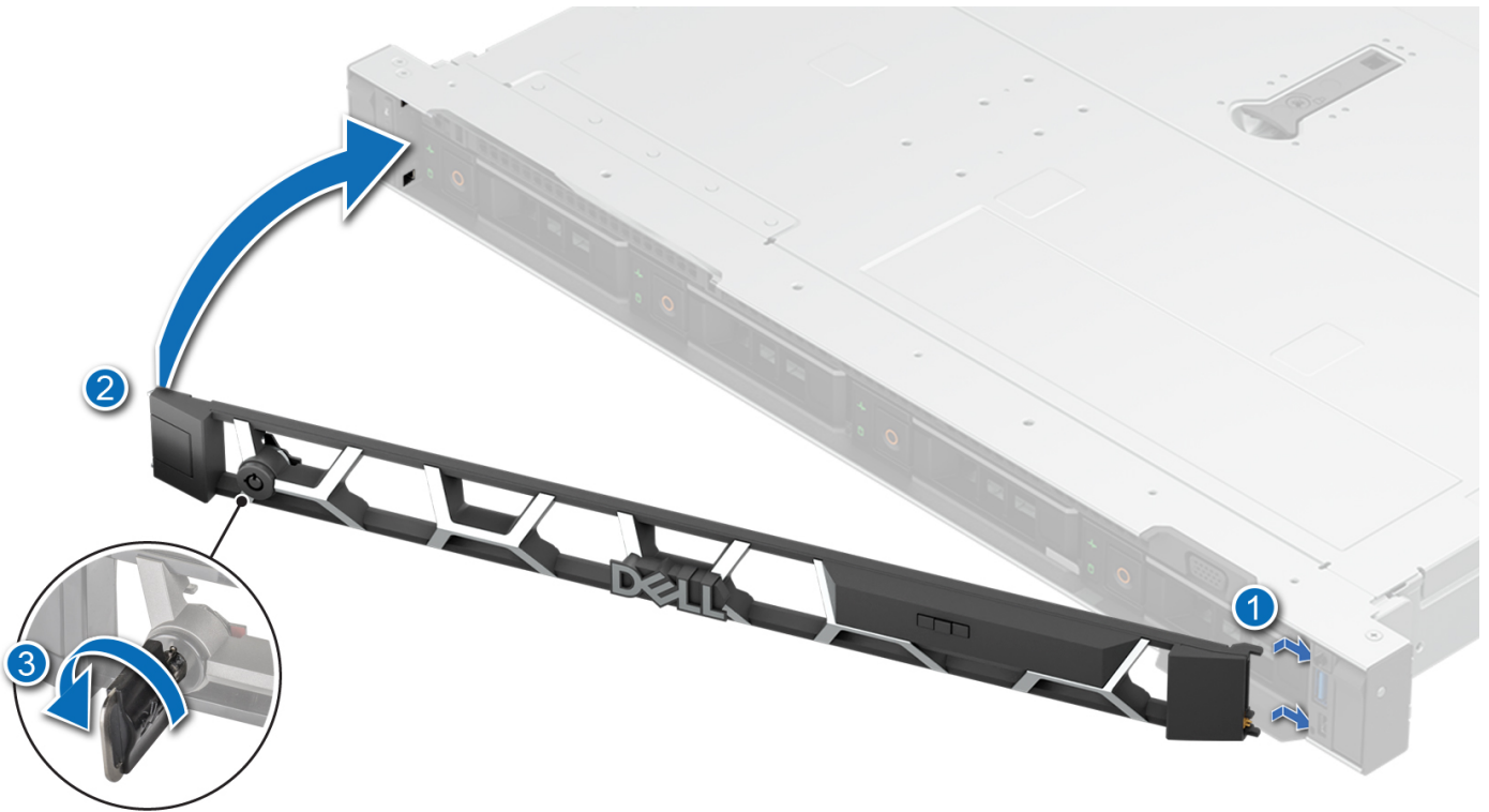
Figure 30. Installing the front bezel
