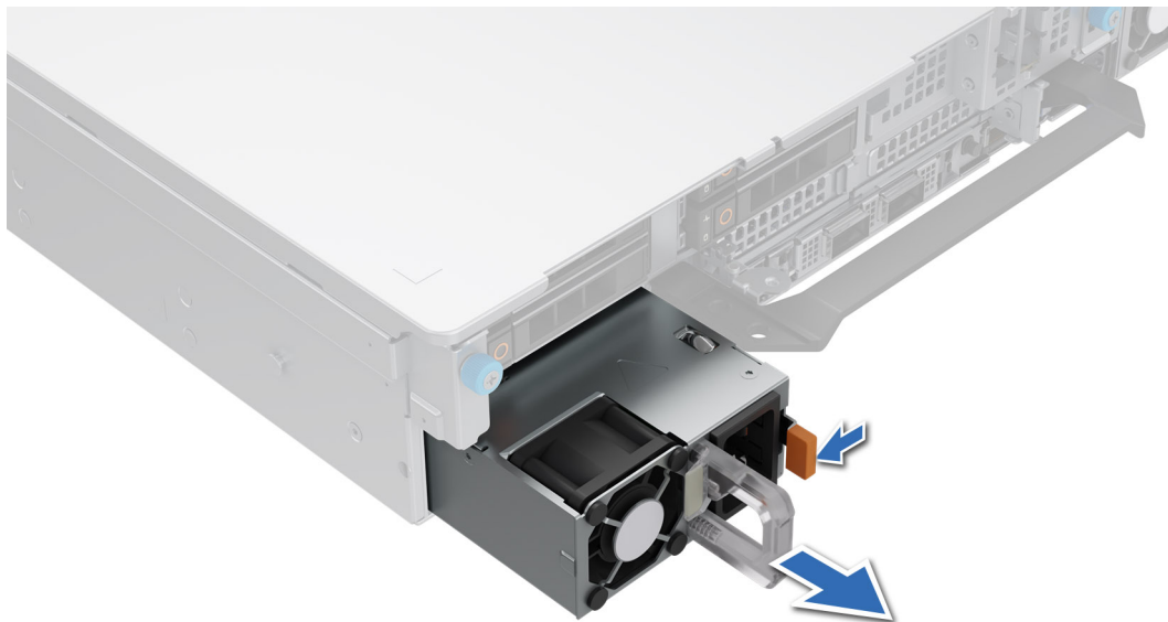
Figure 177. Removing a power supply unit
