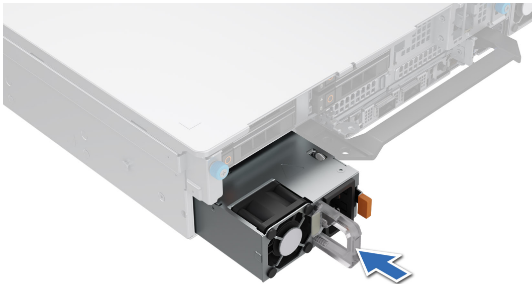
Figure 178. Installing a power supply unit
