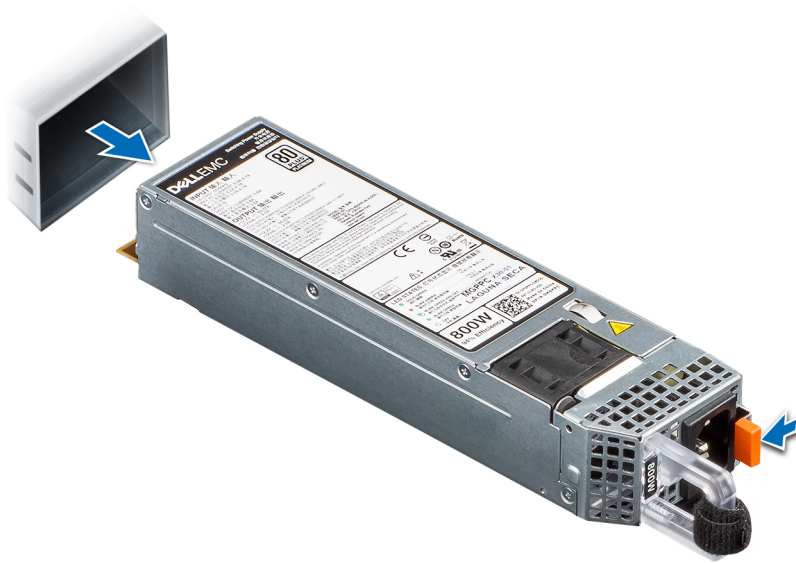
Figure 126. Removing a power supply unit
