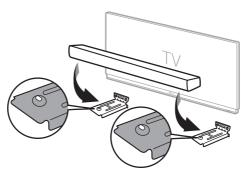
8 Firmly attach the product to the wall brackets using the screws provided.
