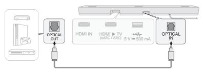
2 Press the Function button repeatedly until "OPT/HDMI ARC" appears on the status display.
