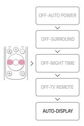
While the "AUTO-DISPLAY", "ON-DISPLAY" or "OFF-DISPLAY" is scrolling in the status display, Press Up/Down button to change the Display to "AUTO" or turn it on or off.
