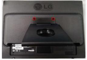
Overturn the set and disassemble the latches of three edges
