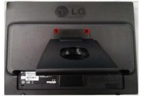
Overturn the set and disassemble the latches of three edges
