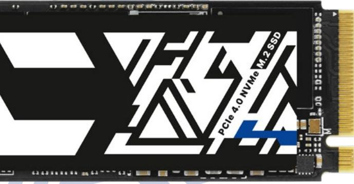
The drive is based on brand-name components, and its efficient operation is supported by the controller, among other things. The reliable PHISON PS5018-E18 controller is a modern solution for fourth-generation SSDs. It provides high performance, stability and data security. The controller supports the PCIe 4 x4 interface and NVMe 1.4 protocol which enables read and write speeds of up to 7 GB/s and as many as 700,000 random IOPS.
