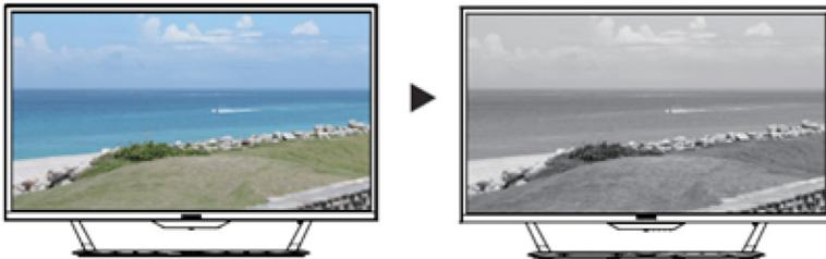
8. Gamma mode allows you to adjust the luminance tone. The default value is 2.2 (standard value for Windows). Adjust range are 1.8, 2.0, 2.2, 2.4 or 2.6.
