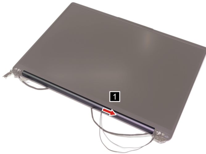
Figure 43. Remove the hinge cover
