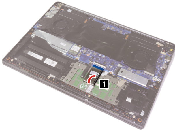
Figure 28. Peel back the keyboard cable
