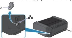
2. Connect the printer and a network device (router, etc.) with an Ethernet cable (A). Do not connect it to the USB port.
